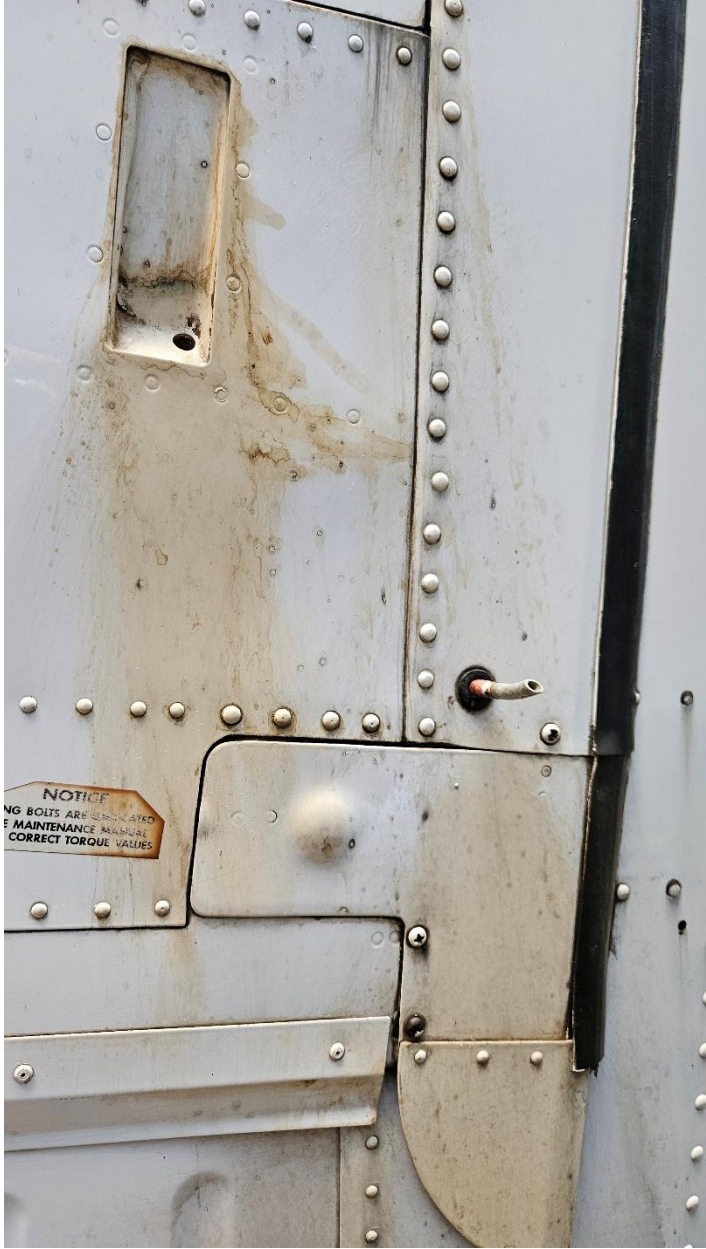
This is the corresponding fuel vent on the other wing. The same degradation pattern is noted.
